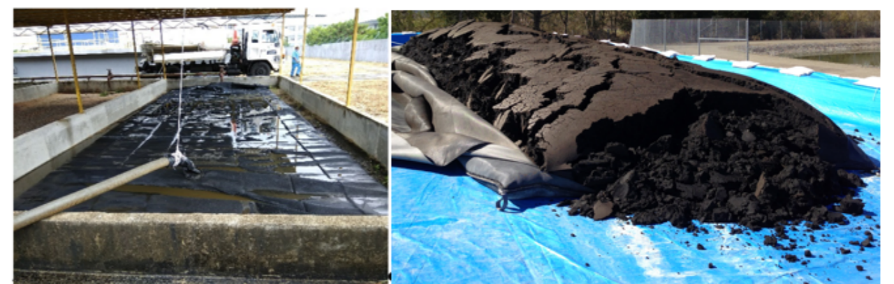
Figure 42: Use of Geotubes for solid liquid separation.
